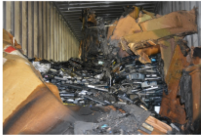
Burnt lithium batteries in fiberboard boxes.
